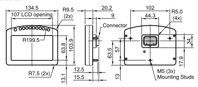
Note: Do not remove any part of the casing. The case provides electromagnetic screening to avoid interference with other equipment, and is also essential for thermal management. Thermal management may be compromised if mounted in a confined space, refer to the operating temperature specifications.
