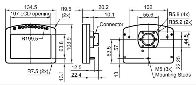
Note: Do not remove any part of the casing. The case provides electromagnetic screening to avoid interference with other => equipment, and is also essential for thermal management. Thermal management may be compromised if mounted in a confined space, refer to the operating temperature specifications. Ensure product is not stressed when mounted.
