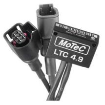
MoTeC's LTC (Lambda To CAN) monitors, controls and diagnoses a Bosch LSU 4.9 Lambda sensor, and transmits Lambda readings on a CAN bus. When using LTCs, up to 32 Lambda sensors can be configured on a single CAN bus allowing an ECU or logging device to simultaneously monitor multiple Lambda sensors.
