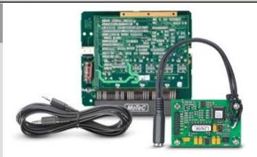
MoTeC's Onboard Knock Module (OKM) enables individual cylinder closed loop knock control on our M800 Plug-In ECUs. The knock module allows tuners to safely optimise high performance ignition maps.
