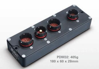
*MoTeC*'s new PDM16 and PDM32 Power Distribution Modules replace conventional relays, fuses and circuit breakers by providing electronically switched power to the various electrical systems in the vehicle, including motors, lights, solenoids and electronic devices such as ECUs and data systems. This simplifies wiring and switch requirements, while increasing reliability.
